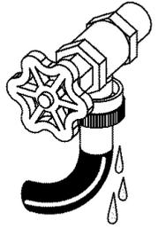
2. Remove the inlet hoses and rubber washers from the plastic bag located in the drum of the washer and install the rubber washers in each end of the inlet hoses.
