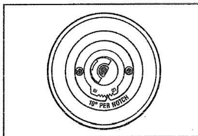
1. Pull off knob. Loosen both screws on back of knob.
