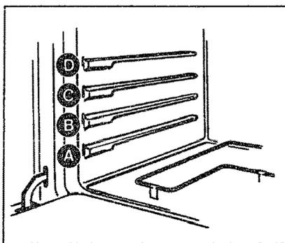
The oven has four shelf supports—**A** (bottom), **B**, **C** and **D** (top). Shelf positions for cooking food are suggested on Baking, Roasting and Broiling pages.
