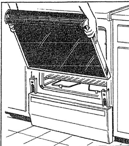
To REMOVE door, open to BROIL position, or where you feel hinge catch slightly. Grasp door at sides; lift door up and away from hinges.
