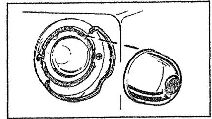
The oven lamp (bulb) is covered with a glass removable cover which is held in place with a bail-shaped wire. Remove oven door, if desired, to reach cover easily.
