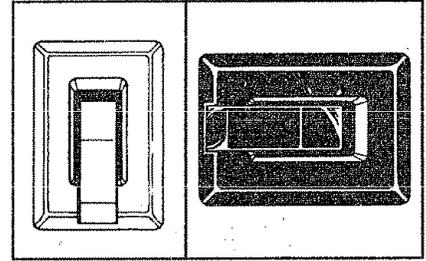
The light comes on automatically when the door is opened. (On models with oven window, use switch to turn light on and off when door is closed.)
