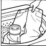
top row of holes. Load evenly to maintain washer balance. Mix large and small items. Items should move easily through the wash water. Overloading can cause poor cleaning. To reduce wrinkling
