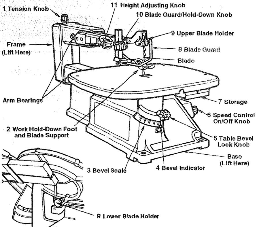
1. **Tension Knob** - Tightening the knob (clockwise) will increase the tension on the blade. Loosening it (counterclockwise) will decrease the tension.
