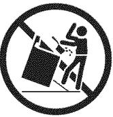
**⚠ WARNING** Stepping, leaning or sitting on the doors or drawers of this range can result in serious injuries and also cause damage to the range. Do not allow children to climb or play around the range. The weight of a child on an open door may cause the range to tip, resulting in serious burns or other injury.
