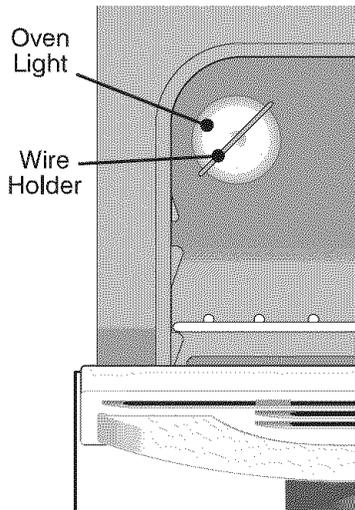
The oven light automatically turns ON when the door is opened. The oven light may also be manually operated by pressing the Oven Light switch located on the upper left control panel.
