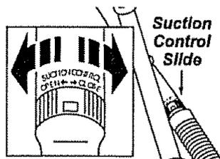
If cleaner has poor cleaning performance, check to make sure the suction control slide is closed.
