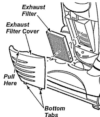
Remove the exhaust filter cartridge.
