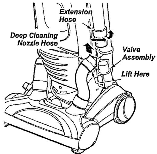
To clean the sensor, remove deep cleaning nozzle hose at valve assembly by lifting hose straight up. Remove extension hose from the valve assembly by grasping hose collar, twisting, and pulling straight off.
