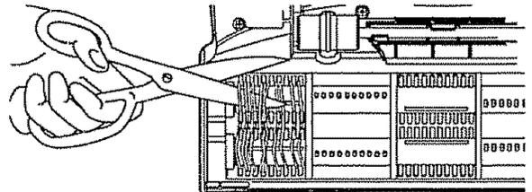
To clean agitator turn vacuum over, cut off any carpet pile and lint entangled around agitator with a pair of scissors in the slots provided. Remove hair, string, lint and other debris from the agitator.
