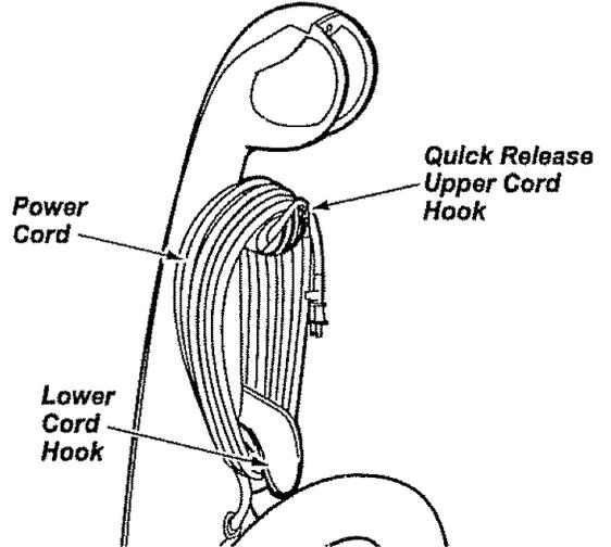
Wrap the power cord around the upper and lower cord hooks and lock the power cord plug onto the power cord.
