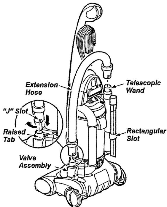
Once extension hose is connected to the telescopic wand, place the wand in the telescopic location as shown.
