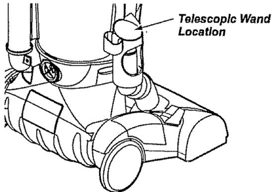
Remove the Handi-Mate Jr. ® from the plastic bag and insert Handi-Mate Jr. ® into the vacuum cleaner as shown, then close the Handi-Mate Jr. ® storage cover.
