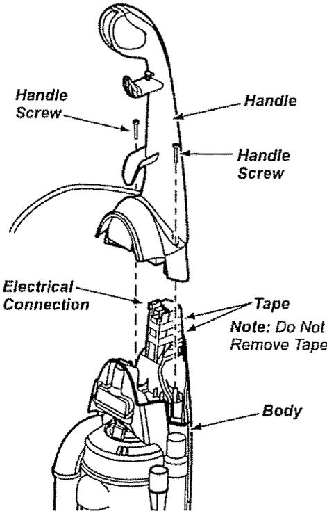
When installing the handle, firmly press the handle onto the body. Secure with handle screws provided.
