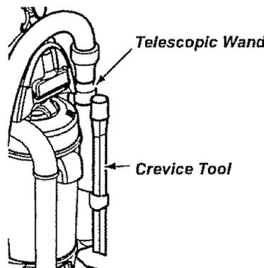
Remove the telescopic wand from its storage position by twisting and pulling out.
