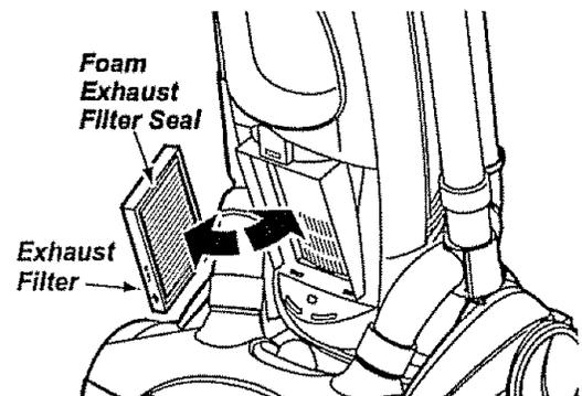
The foam seal of the filter should be placed against the vacuum cleaner body
