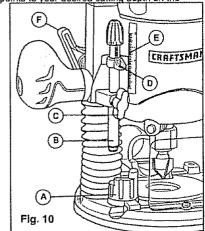
NOTE: When making depth adjustments on the plunge base, the motor clamp should always be closed securely.
