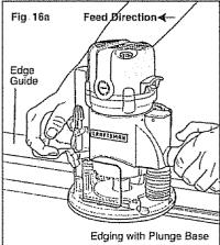
⚠ WARNING: Always securely clamp your workpiece and keep a firm grip on the router base with BOTH HANDS at all times. Fallure to do so could result in loss of control causing possible serious personal injury.
