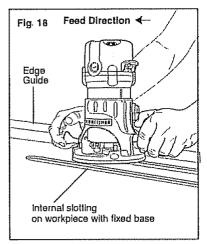
MARNING: Always securely clamp your workplece and keep a firm grip on the router base with BOTH HANDS at all times. Failure to do so could result in loss of control causing possible serious personal injury.
