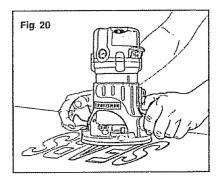
NOTE: A core box or V-groove bit is often used for routing letters and engraving objects. Straight bits and ball mills are often used to make relief carvings. Veining bits are used to carve small, intricate details.
