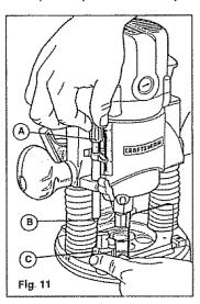
Always set your micro adjustments with the plunge action in the RAISED, (or up) position, and locked down.
