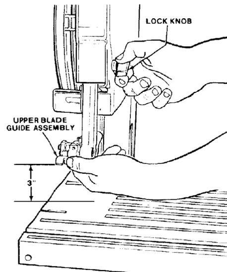
3. Loosen the two capscrews that lock the upper blade guides using a 1/8-inch hex "L" wrench and separate them about 1/8-inch. Repeat the same step for the lower blade guides.
