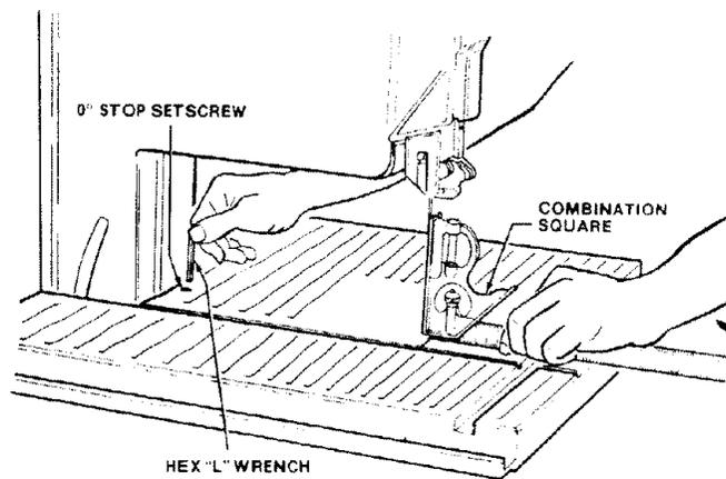
to set the 0° stop. Turn screw until it makes contact with the frame.
