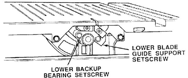
**CAUTION:** Do not use the metal blade guides supplied with your band saw when using the 1/16-inch blade. The metal blade guides must be removed. Use only the non-metallic blade guides supplied with the 1/16-inch scroll cutting band saw blade.
