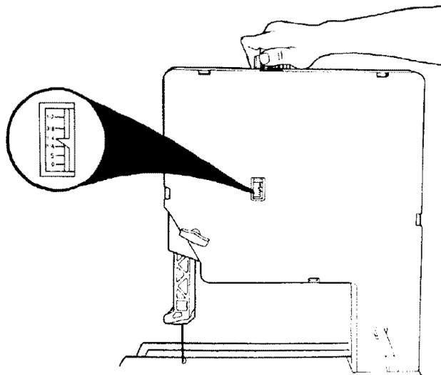
2. Turn the upper wheel by hand a few times and notice if the blade remains in the center of the tire on the top wheel.
