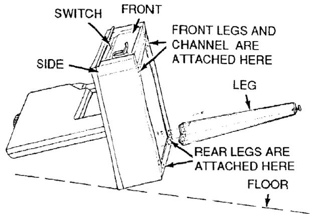
3. Mount the two *front* legs to the basic saw assembly using truss head bolts, lockwashers, and nuts. Make sure that the four (4) holes in each corner of the saw line up with the four (4) holes in the top of each leg. At this time only put bolts through the *sides* of the saw assembly *not* the front. Only fingertighten nuts.
