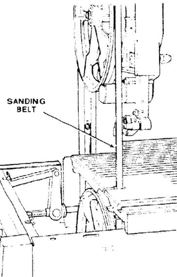
**NOTE:** A new sanding belt will stretch with use, so check the tension often.
