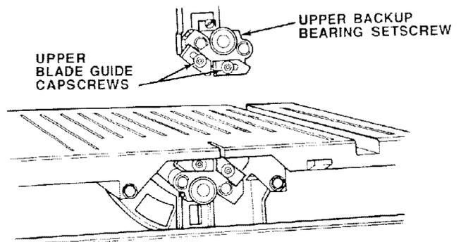
5. Locate the special blade guides that are supplied with the 1/16-inch blade. Remove the blade guides and separate as shown. Discard center piece and plug. Inspect blade guides for burrs and if present remove with fine sandpaper.
