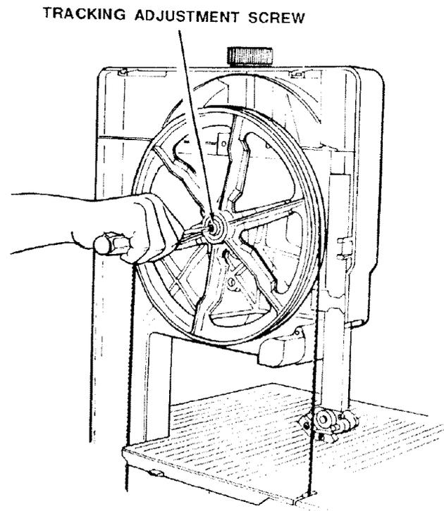
**NOTE:** Because of manufacturing tolerances in band saws and blades, it may be difficult to track the blade in the center of the wheel. The blade may exhibit a tendency to wander to the front of the wheel. If this condition exists, track the blade on the back half of the upper wheel.
