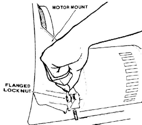
1. Install the wing nut on the threaded stud.
