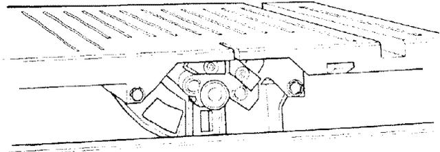
4. Slide the sanding platen into the blade slot in the table and fasten to the upper blade guide assembly where the right blade guide mounts. It may be necessary to loosen the left blade guide and slide it backwards until platen is in place.
