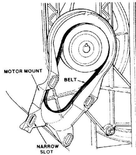
7. Carefully position the motor so that the poly "V" belt is around the motor pulley and the four motor studs align with the slots in the motor mount.
