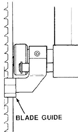
turning. If the bearing is turning, the blade is too close. Move bearing slightly away from blade and tighten set screw with 1/8-inch hex "L" wrench. Turn upper wheel and recheck
