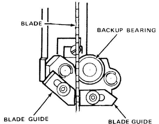
6. To insure the backup bearing is properly supporting the blade, push the bearing toward the blade until it almost touches it. Turn the upper wheel, by hand, checking the backup bearing to make sure it is not turning. If the bearing is turning, the blade is too close. Move bearing slightly away from the blade and tighten set screw with 1/8" hex "L" wrench. Turn upper wheel and recheck the bearing. Adjust again if necessary.
