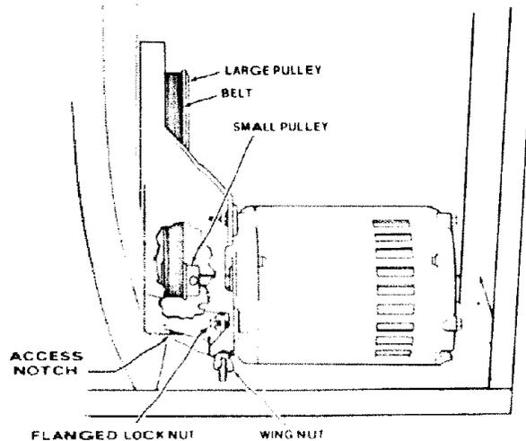
4. Belt tensioning is done by tightening the wing nut which pulls the motor down. The motor slides on the three (3) spacers and is locked in place by the flanged lock nuts on the threaded studs.
