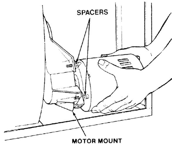
9. Install the threaded stud through the hole in the lower leg of the motor mount and over the motor stud as shown.
