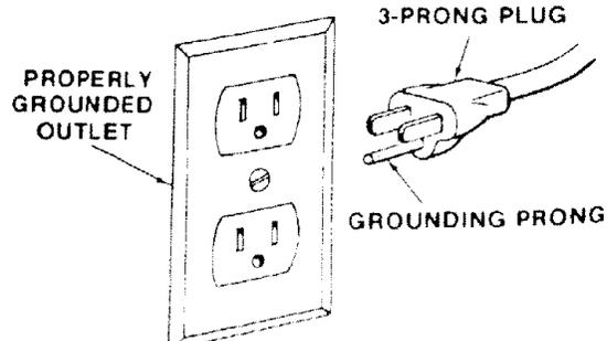
This power tool is equipped with a 3-conductor cord and ground type plug listed by Underwriters' Laboratories. The ground conductor has a green jacket and is attached to the tool housing at one end and to the ground prong in the attachment plug at the other end.
