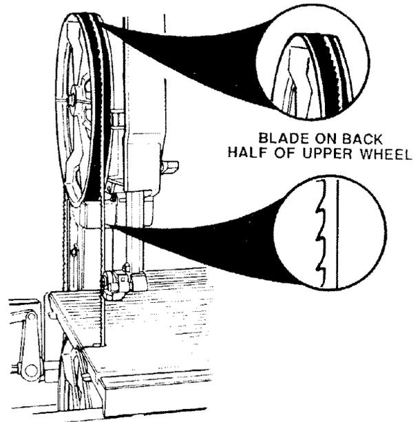
10. Push the blade guide support toward the blade and adjust the blade guides so they are even with the front edge of the blade.
