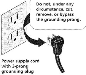
Power supply cord with 3-prong grounding plug
