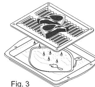
**Note:** The broiler pan and the insert allows grease to drain and be kept away from the high heat of the broiler (See Fig. 3). **DO NOT** use the pan without the insert. **DO NOT** cover the insert with foil; the exposed grease could ignite.
