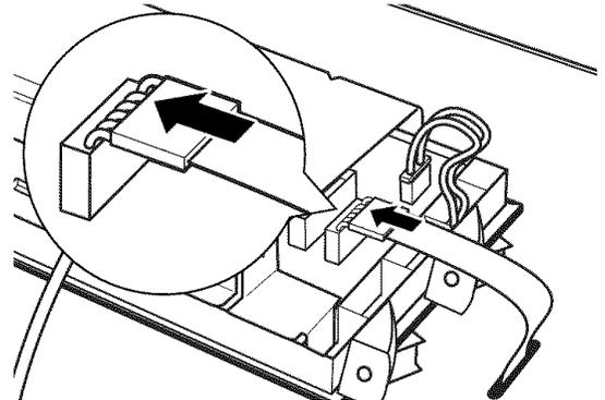
Place the ribbon and the wire from the rear cover under the strain relief on the new backsplash.
