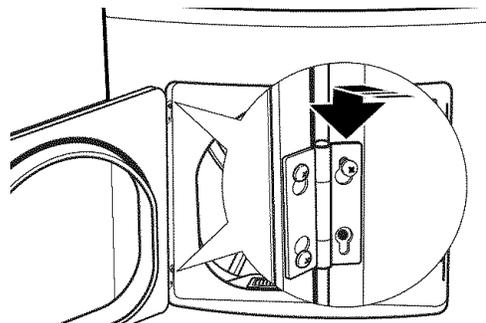
Remove the remaining screws from the side of the opening from which the door was removed. With these screws, secure each hinge at the bottom.
