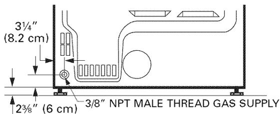
**NOTE:** Add to vertical dimension the distance between cabinet bottom to floor.
