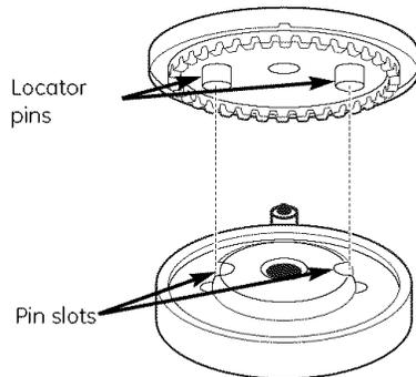
When placing, make sure the locator pins in the burner head are seated in the pin slots of the burner base. Rotate the burner head around the burner base until it is level and securely seated.
