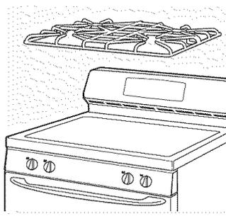
Lift out when cool. Grates should be washed regularly and, of course, after spillovers. Wash them in hot, soapy water and rinse with clean water. When replacing the grates, be sure they are positioned securely over the burners.
