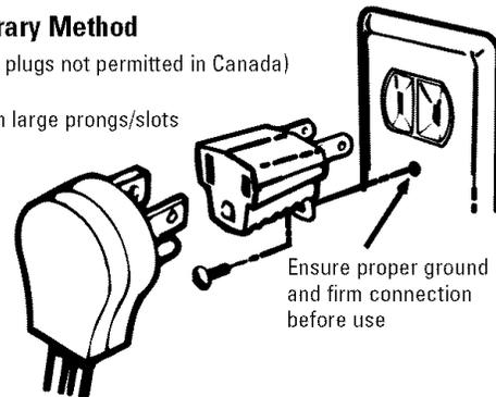
Ensure proper ground and firm connection before use
