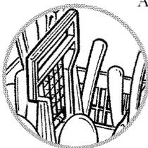
A security cell cover (on some models) hinged in some handles can be lowered to either side to secure lightweight items from the effects of the vigorous wash action.
