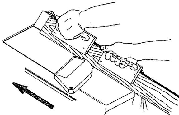
Use hold down/push blocks for wood under 3 in. wide. Position them so you have control of the work piece at all times and so they do not contact the guard or the cutter head.
