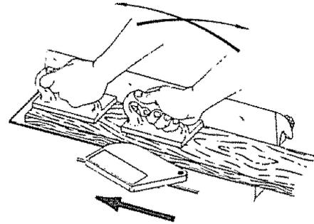
This means that once the work piece has passed the cutter head onto outfeed table, one hold down/push block must always maintain contact with the work piece with outfeed table.
