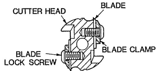
NOTE: Check blade height at both ends of blade. After the first one is adjusted, repeat for second blade.
