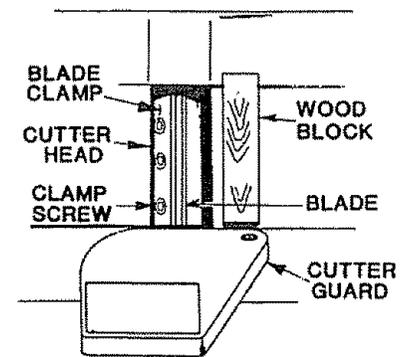
2. Locate the slot in the cutter head shaft through the small hole in the backside of the machine directly above the vacuum port. Rotate the cutter head with a screwdriver until one of the blades is at its highest position.
