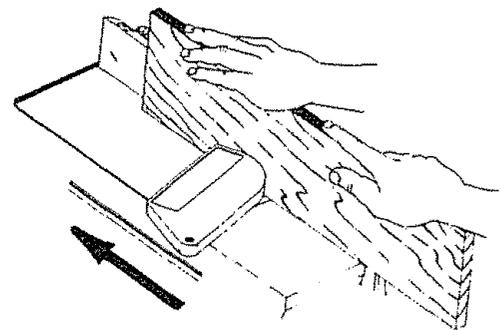
Always feed **WITH THE GRAIN** whenever possible. If the nature of the work piece is such that it must be fed **AGAINST THE GRAIN**, take very light cuts and feed slowly.
