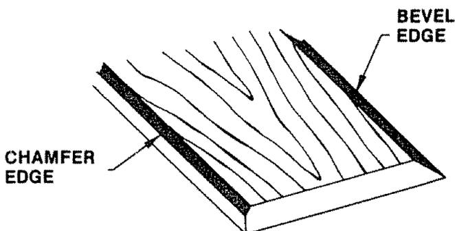
**CHAMFERING** is removing only the corner of the edge of a board. Normally a chamfer is made with one cut; therefore, a cut deeper than 1/16" may be made.
