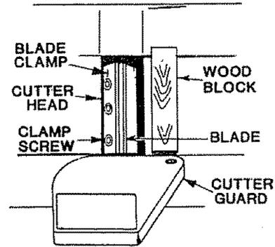
5. Clean any sawdust from cutterhead and any parts you have removed.
