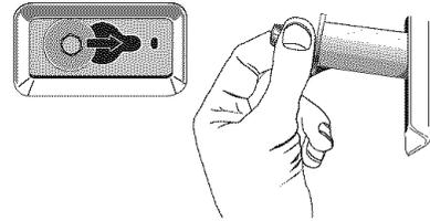
3. Once all 4 bolts are removed, discard the bolts and spacers. Then pull the power cord through the opening of the rear panel and close the hole with the attached cap.
