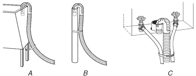
If the washer faucets and the drain standpipe are recessed (see illustration C), put the hooked end of the drain hose in the standpipe. Tightly wrap the cable tie around the water inlet hoses and the drain hose.
