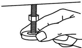
4. Check the levelness of the washer by placing a level on the top edge of the washer, first side to side, then front to back.
