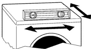
5. Rock washer gently front to back, side to side and diagonally to make sure that all four feet are in firm contact with the floor.
