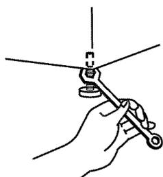
**IMPORTANT:** All four feet must be tightened. If the nuts are not tight against the washer cabinet, the washer may vibrate.
