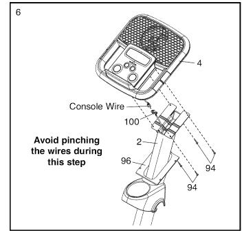
7. Slide the Console Cover (96) (see the drawing in step 6) upward to the Console (4). Attach the Console Cover with four M4 x 16mm Screws (84).
