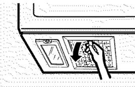
**To remove**, slide it to the rear using the tab. Pull it down and out.
