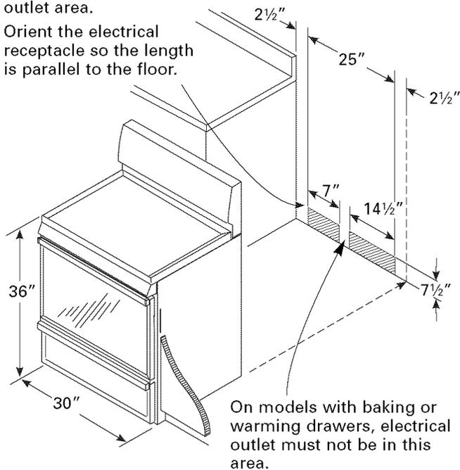
**NOTE:** Use a 4' power cord to prevent interference with the storage drawer. Power cords 4½ to 6' long may have to be dressed to allow for proper drawer closing.
