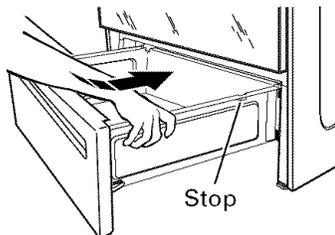
**C** Lift the front of the drawer and push in until the stops clear the guides.
