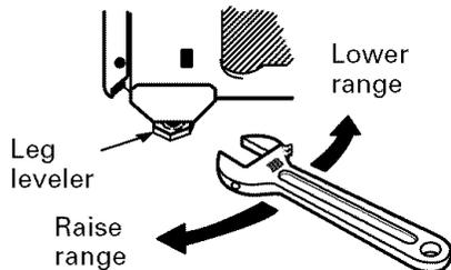
**D** Use an open-end or adjustable wrench to adjust the leveling legs until the range is level.
