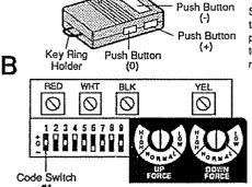
Select a transmitter push button to operate receiver
