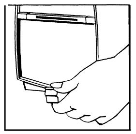
To remove wheeled carrier, depress metal clip at small wheel end while lifting up cleaner.
