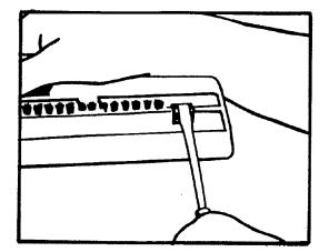
2. Screw springs onto projections of new brush. Center new brush in nozzle. Make sure that the bristles are facing up and the projection side is turned toward tube. Replace the clip and clamp into position by pressing down with the flat side of a screwdriver.
