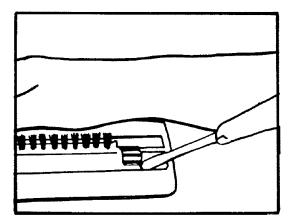
1. Remove one of the metal clips holding brush in position by placing a screwdriver under the raised edge and lifting upward. Note position of old brush and springs, then remove them.
