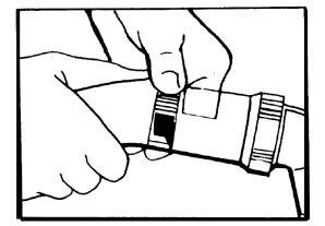
On certain types of dense carpet, it may be advantageous to keep the brush in a position where it does not come in contact with the carpet. To lock brush into the nozzle, adjust lever to "RUG" position then press the brush all the way into the nozzle with your finger. While still holding the brush, adjust the lever to the "FLOOR" position and the brush will be locked into place. To release brush; move the brush lock lever either to the left or right to the "RUG" position.
