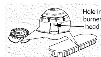
The oval burner head/cap assembly is removable. Simply lift it off the range for cleaning. Use a sewing needle or twist-tie to unclog the small hole in the burner heads.
