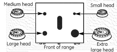
Make sure the slot in the burner head is positioned over the electrode.
