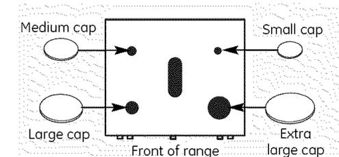
Make sure that the heads and caps are replaced in the correct locations.
