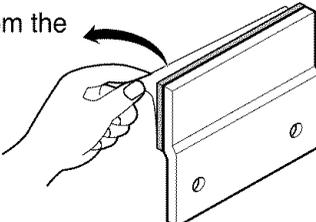
**4** Attach the double-faced tape of the bracket to the dryer as shown so the bent parts of the brackets align with the edge and can be attached to the pedestal with screws.
