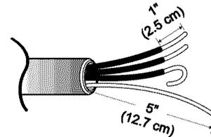
Then, put the hooked shape end of the wire under the screw of the terminal block(hooked end facing rightward) and pinch the hook together and screw tightly.
