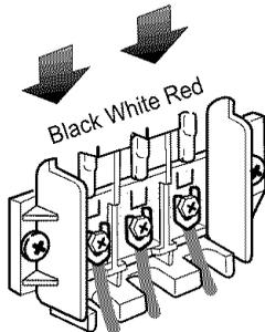
1. Connect neutral wire(white) of power cord to center terminal block screw.
