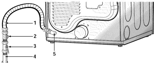
1. New stainless steel flexible connector. Use this type of connector only if allowed by local codes. Use Design AGA Certified Connector.
