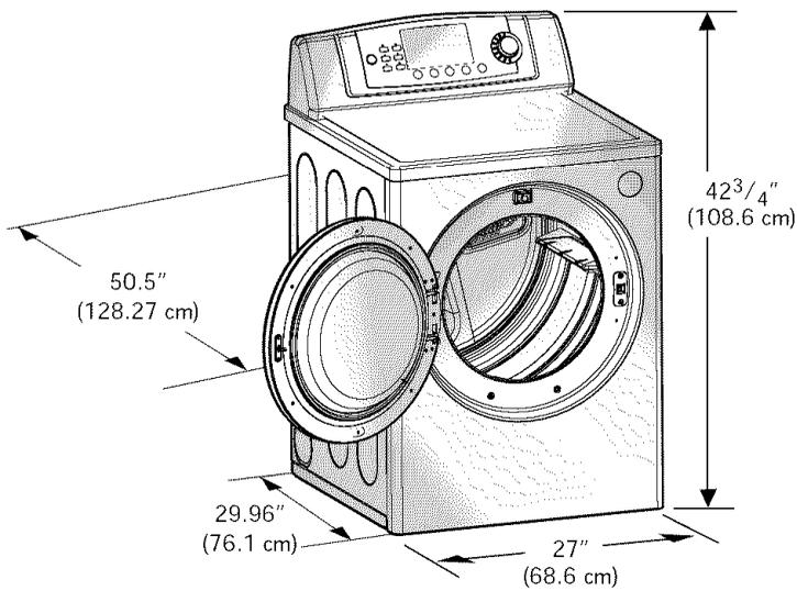
\* Most installations require a minimum 5 1/2 in. (14 cm) clearance behind the dryer for the exhaust vent with elbow.
