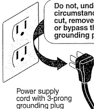
Power supply cord with 3-prong grounding plug
