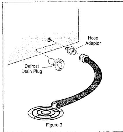
Defrost water will drain out. Check pan occasionally so water does not overflow. Replace the drain plugs when defrosting is completed.
