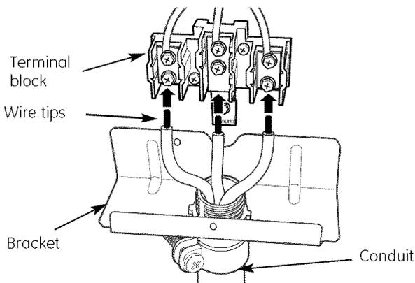
Wire used, location and enclosure of splices, etc., must conform to good wiring practices and local codes.
