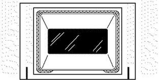
The gasket is designed with a gap at the bottom to allow for proper air circulation.
