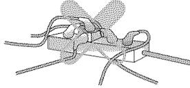
**Do not allow the power plug to face upward or to be squeezed at the back of the refrigerator.**
