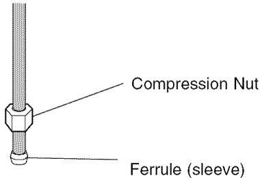
2. Insert the tube into the valve and fasten with wrench as shown in the figure below.
