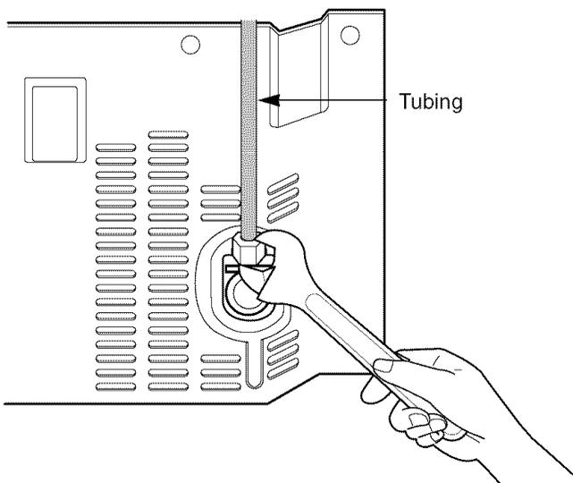
**CAUTION** Check to see if leakage occurs at water line connections.
