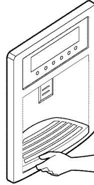
Tilt up the front of the tray slightly and snap the ribs into the holes to reinstall the tray.
