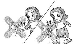
**Remove water or dust from the power plug and insert it with the ends of the pins securely connected.**
