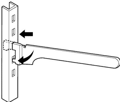
Then lower the front of the shelf so that the hooks drop into the slots.
