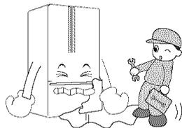
**Do not install the refrigerator in the wet place or the place which water or rain splashes.**
