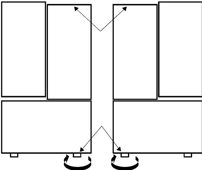
3. Open both doors again and check to make sure that they close easily. If not, tilt the refrigerator slightly more to the rear by turning both leveling legs clockwise. It may take several more turns, and you should turn both leveling legs the same amount.
