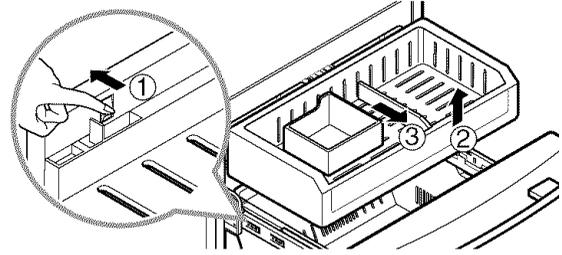
To install, after pulling out both rails as much as possible, and gently push down both left and right side while checking the hook on the front part.
