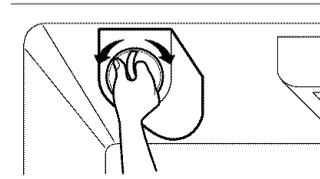
If you can't turn the filter from side to side, it isn't fully inserted. Push it in firmly and twist it into place. You will hear the snap when it clicks into place.
