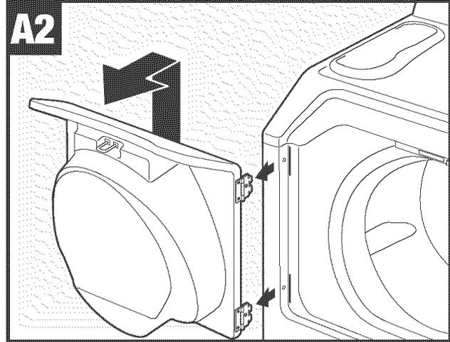
Remove door by lifting up then out to disengage hinges from washer./Enlevez
