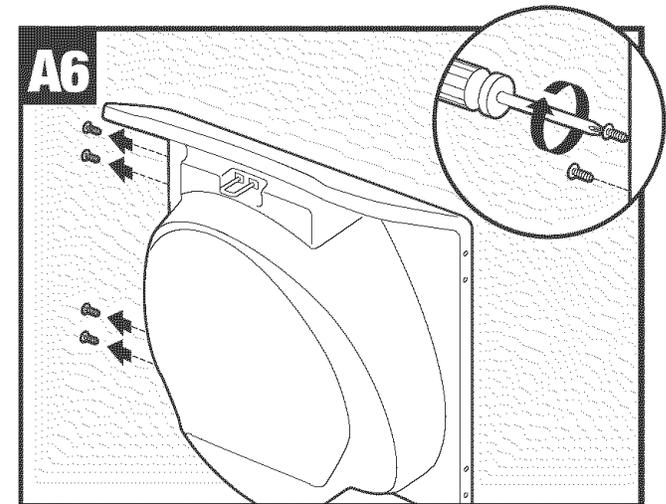
Remove the four color-matching screws from the opposite edge of door./Retirez les
