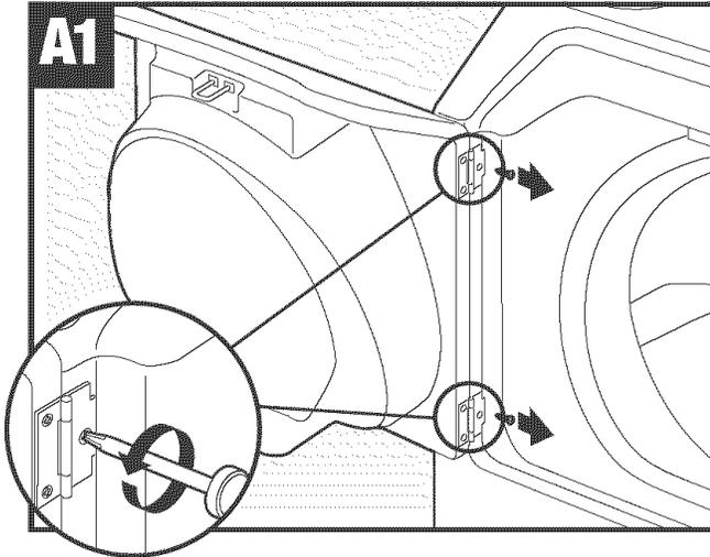
Remove center screws from hinges./Retirez les vis centrales des charnières./
