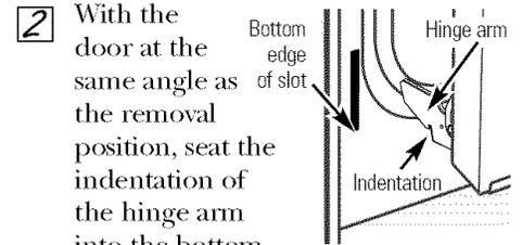
2 With the door at the same angle as the removal position, seat the indentation of the hinge arm into the bottom edge of the hinge slot. The notch in the hinge arm must be fully seated into the bottom of the slot.
