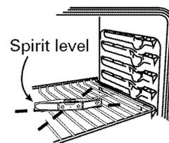
**C** On all models except warming drawer models, remove the storage drawer, broiler drawer or kick panel. The front leveling legs can be adjusted from the bottom and the rear legs can be adjusted from the top. (For warming drawer models, see Step D.)
