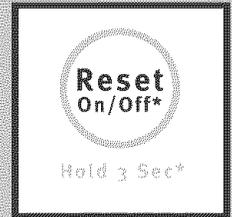
Once you disable the alarm system, you must again press *and hold* the **Alarm Reset** button for three more seconds to reset (activate) the alarm system. The **On** indicator light remains off while the Freezer and Fresh Food compartments cool toward the current temperature settings. When temperature settings are reached, the **On** light displays green to indicate an active alarm system.
