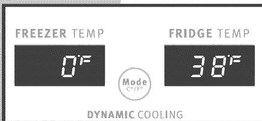
The two digital displays on the left half of the control panel indicate the current temperatures of your freezer and fresh food compartments.
