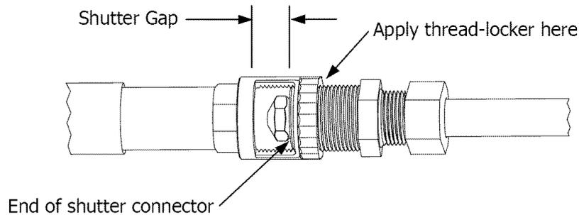
**Figure 9-2 Air Shutter Reassembly and Gap Adjustment**
