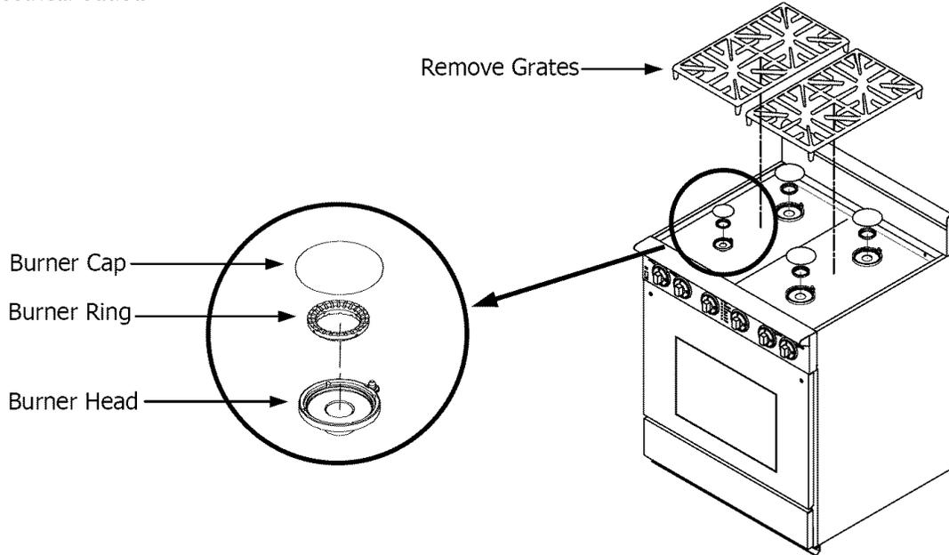
**Figure 3-1 Grate, Burner Cap and Burner Ring Removal**
