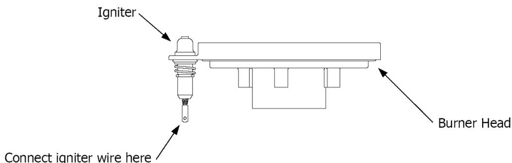
**Figure 10-1 Igniter Connection**
