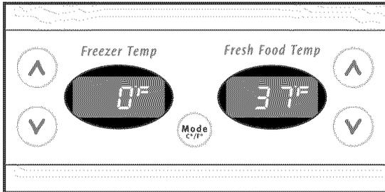
To adjust the temperature to a higher or lower setting, press the **Up (Cold)** or **Down (Colder)** button closest to the display. The first time you press the button, the display shows current setting you entered. Each press of the button after that changes the setting by one degree.
