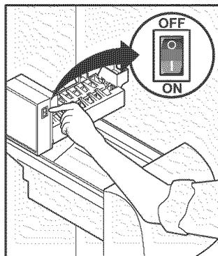
to the ice maker, pull the ice cream tray out. Press the switch to the "O" position to turn it Off and press it to the "I" position to turn it On. With no usage it will take approximately 2 days to fill the ice container. The ice maker also has a built-in wire signal arm, which automatically stops ice production when the ice bin is full. This signal arm should not be used to manually stop the ice maker.
