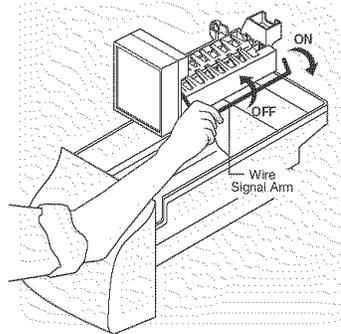
The ice maker turns off automatically when the ice container becomes full. To stop the ice maker, lift the wire signal arm until it clicks, and locks in the "up" or OFF position.
