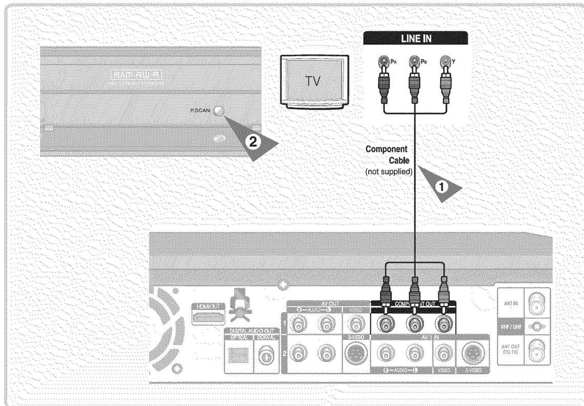
1. Connect the Component video cables(not supplied) between the COMPONENT OUT(Y,P<sub>B</sub>,P<sub>R</sub>) jacks on the DVD Recorder and COMPONENT IN(Y,P<sub>B</sub>,P<sub>R</sub>) jacks on your TV (or AV amplifier).
