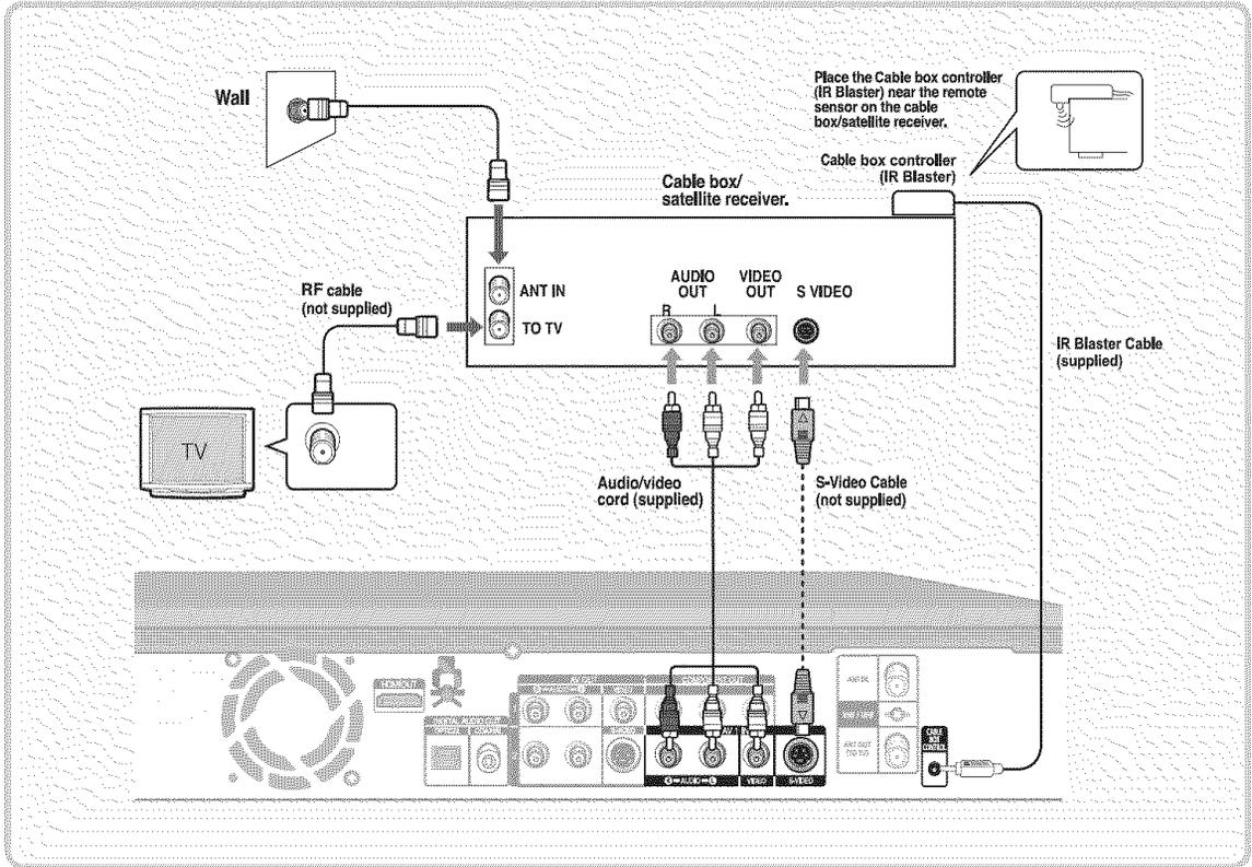
**Connecting the IR Blaster cable into the Cable Box Control jack**
