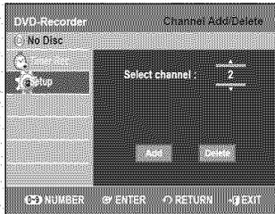
*Manual Channel Set can be used after you have first performed Auto Channel Memory. Use the Manual Channel Setting to delete unnecessary channels.*
