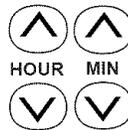
The **HOUR/MIN UP** and **DOWN** arrow pads set the time of day, length of cooking time, length of cleaning time, the delayed start time, and the time set on the Kitchen Timer.
