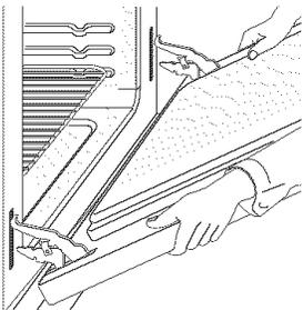
HINGE SLOT - Door removed
