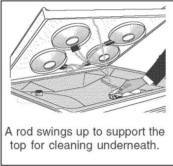
A rod swings up to support the top for cleaning underneath.
