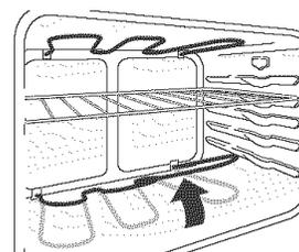
The baking element may be tilted about 4 or 5 inches to clean the oven bottom.
