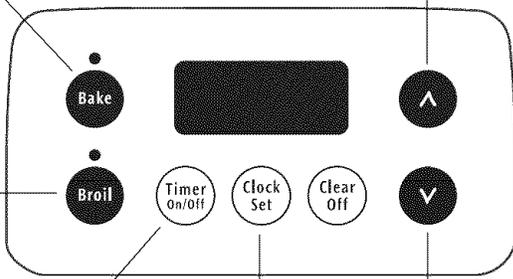
**TIMER ON/OFF PAD**— Used to set or cancel the minute timer. The minute timer does not start or stop cooking.
