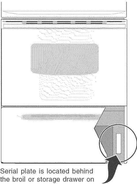
Serial plate is located behind the broil or storage drawer on the lower right side of the appliance frame.
