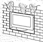
Leave some space around the TV set as shown below. Otherwise, air-circulation may be inadequate and cause overheating, which may cause a fire or damage to the TV set.
