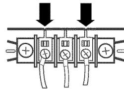
4. Tighten strain relief screws.
