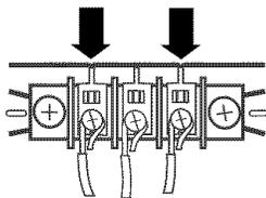
4. Tighten strain relief screw.
