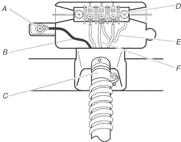
A. External ground conductor screw
