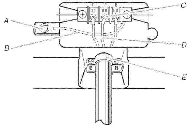
A. External ground conductor screw
