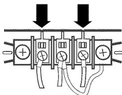
5. Tighten strain relief screws.
