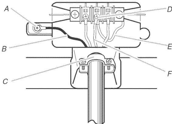
A. External ground conductor screw
