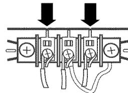
4. Tighten strain relief screws.
