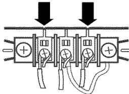
5. Tighten strain relief screw.
