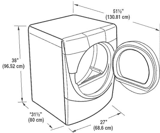
\*Most installations require a minimum 5" (12.7 cm) clearance behind the dryer for the exhaust vent with elbow. See "Venting Requirements."
