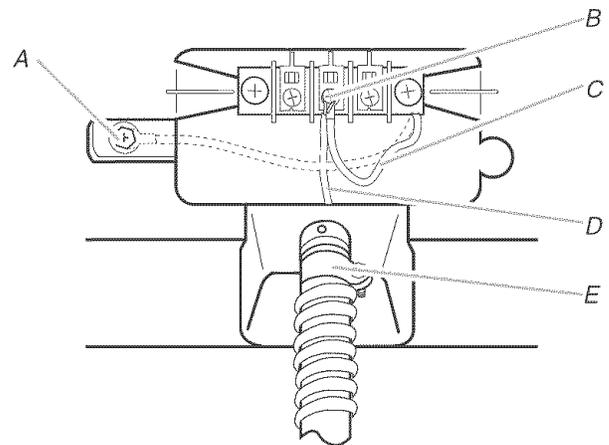
A. External ground conductor screw - Dotted line shows position of NEUTRAL ground wire before being moved to center silver-colored terminal block screw
