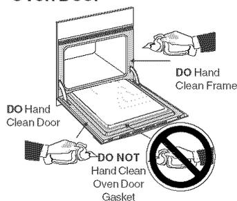
Use soap & water to thoroughly clean the top, sides and front of the oven door. Rinse well. You may use a glass cleaner on the outside glass of the oven door. **DO NOT** immerse the door in water. **DO NOT spray or allow water or the glass cleaner to enter the door vents.** **DO NOT** use oven cleaners, cleaning powders or any harsh abrasive cleaning materials on the outside of the oven door.
