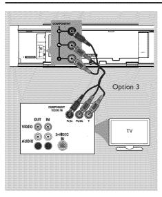
Option 3: Connecting to a Progressive Scan TV or component video input
