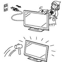
The screen is glass and can be scratched or broken when dropped or impacted.
