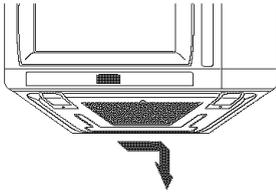
3. Soak grease filter in hot water and a mild detergent. Scrub and swish to remove embedded dirt and grease. Rinse well and shake to dry. Do not clean filter with ammonia, corrosive cleaning agents such as lye-based oven cleaners, or place them in a dishwasher. The filter will turn black or could be damaged.
