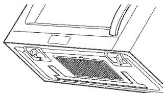
2. Remove the bulb cover mounting screws.
