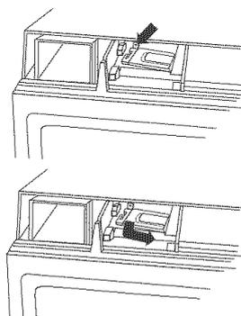
5. Replace bulb with a 30 or 40 watt appliance bulb.
