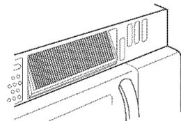
6. Slide the bottom of the grille into place. Push the top until it snaps into place. Replace the mounting screws. Turn the power back on at the main power supply and set the clock.
