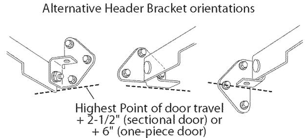
**Figure 18** Attach Header Bracket above Garage Door
