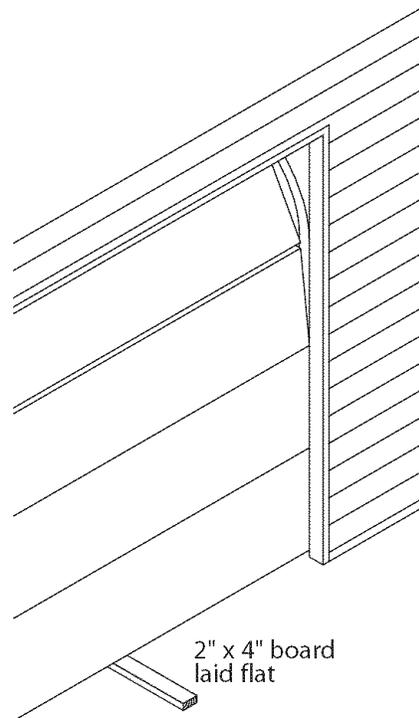
**Figure 36** Checking Contact Reverse
