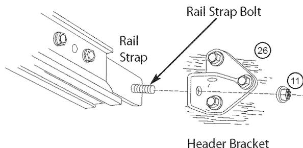
**Figure 20** Attach Rail Strap to Header Bracket
