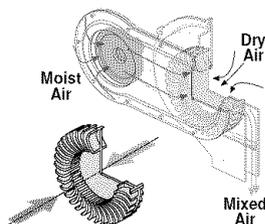
This is one of the best performance solutions for drying dishes because it minimizes venting humid air to the outside of the dishwasher. In addition, this system ensures better drying results compared to the condensing drying system.
