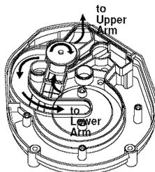
Because of alternating water spray between the Upper and Lower Rack, the water pressure allows superior performance and reduced consumption of water and electricity.
