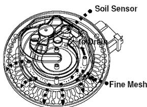
For best wash results, the self-cleaning filter system continuously cleans the water as it circulates. Your LG dishwasher has a self-cleaning filter that grinds food into small particles before it goes down the drain.
