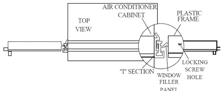
3. Insert top and bottom legs of window filler panel frame into channel in the top angle and bottom rail. Do both sides.
