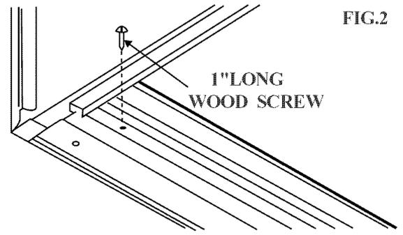
Refer to Step 4 of Window Mounting for assembly of support brackets. A wooden strip nailed to the outside wall should be used in conjunction with sill support angle brackets.
