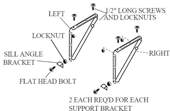
2. Assemble sill angle bracket to support brackets at the marked position, as shown. Hand tighten, but allow for any changes later.
