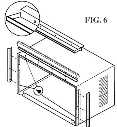
2. Install top angle and side retainers to cabinet as shown in FIG. 6.
