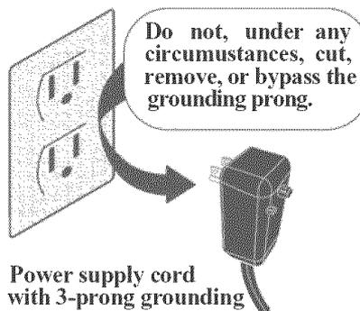
**Do not, under any circumstances, cut, remove, or bypass the grounding prong.**
