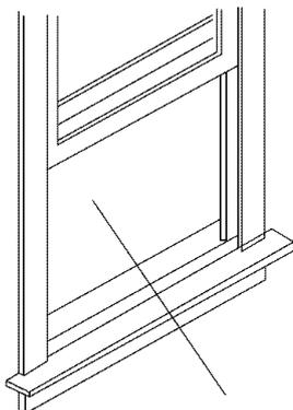
2. Place cabinet in window with bottom stool angle firmly seated over window stool as shown. Bring window down temporarily behind top angle to hold cabinet in place.
