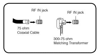
Connect the 75 ohm Cable from the Combination VHF/UHF Antenna to the RF IN Jack.
