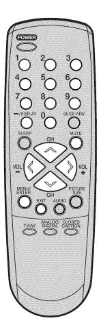
To use the TV after the TV is protected. When a program is received that is blocked by the V-Chip, press MUTE and enter the password, then press MENU/ENTER. When the password is entered correctly the protection will be temporarily overridden.
