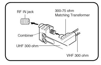
Connect the UHF 300 ohm Twin-lead Wire to the Combiner (not supplied). Connect the VHF 300 ohm Twin-lead Wire to the 300-75 ohm Matching Transformer. Attach the Transformer to the Combiner, then attach the Combiner to the R Jack.
