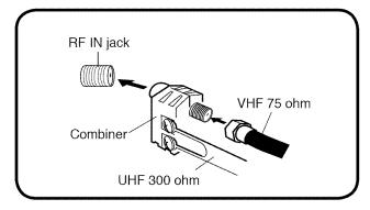
Connect the VHF 75 ohm cable and UHF 300 ohm Twin-lead Wire to the Combiner. Attach the Combiner to the RF IN Jack.
