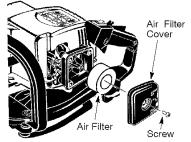
A dirty air filter decreases engine performance and increases fuel consumption and harmful emissions. Always clean after every 5 hours of operation.
