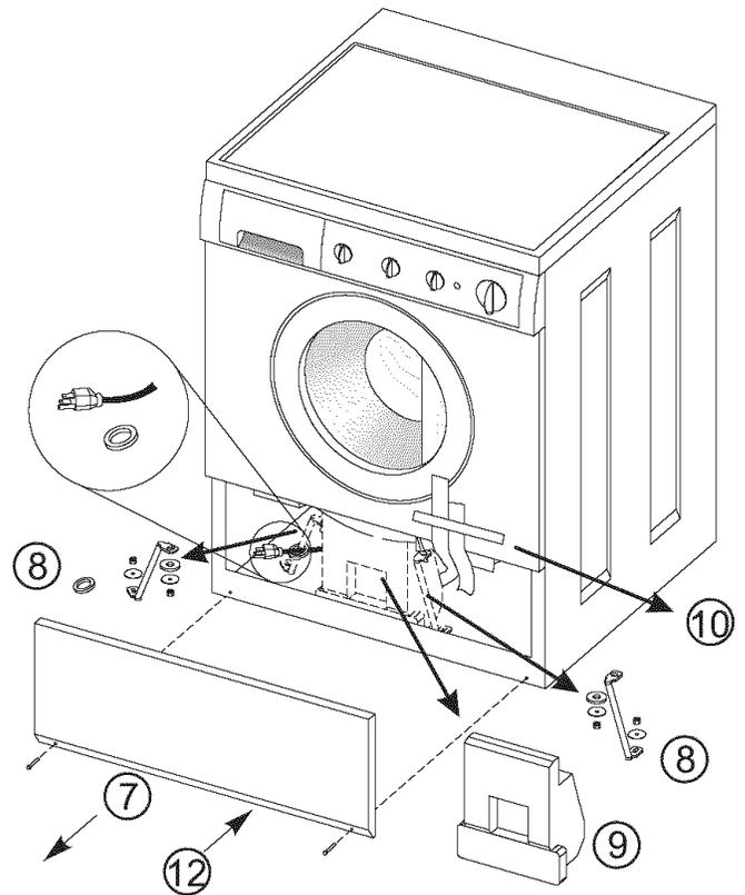
9. Remove the large styrofoam block located under the drum. Lift up on the drum, tilt the base of the foam block inwards toward the rear of the washer until free, then pull it out.
