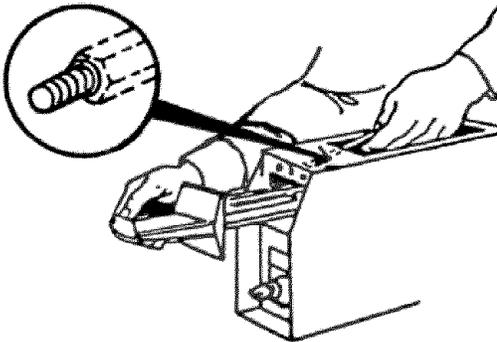
4. While holding the bolt in place, guide the coin slide mechanism onto the threads and into the guide holes in the front of the meter case.
