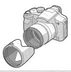
3 Attach the lens hood with the screw facing upwards and then tighten the screw again.
