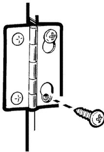
4 Remove the remaining screws from the side of the opening from which the door was removed. With these screws, secure each hinge at the bottom. Tighten the 2 top screws of each hinge. Reinsert the plastic plugs on the side from which the door was removed.
