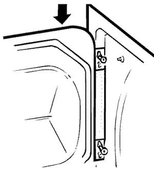
3 Rotate the door 180°. Insert it on the opposite side of the opening by moving the door **IN** and **DOWN** until the top hinge and the bottom hinge are resting on the top screws inserted in step 1.
